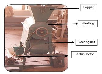
Figure 1. Shea nut shelling machine
